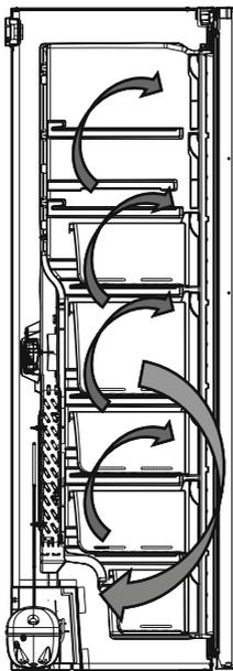
The situation is completely different in no-frost freezers. Dry and cold air is blown into the freezer compartment homogeneously and evenly from several points via a blower fan. Cold air dispersed homogeneously and evenly between the shelves cools all of your food equally and uniformly, thus preventing humidity and freezing.
