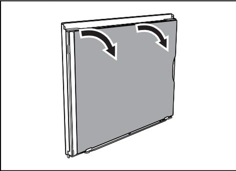
2. Then, pull the glass panel upwards, paying attention to the brackets at the bottom of the door.
