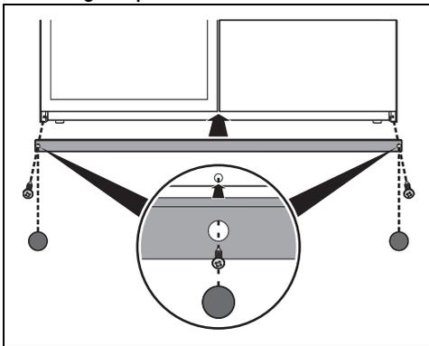
The plinth must always be positioned and secured correctly on the appliance.
