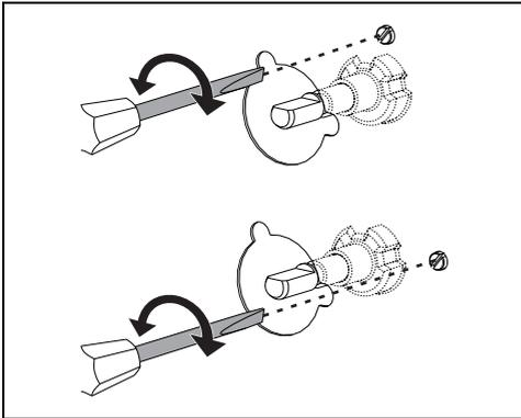
Light the burner and turn it to the minimum position. Extract the gas cock knob and turn the adjustment screw next to the gas cock spindle
