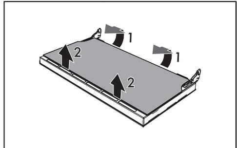
3. Remove the intermediate glass pane by lifting it upwards.
