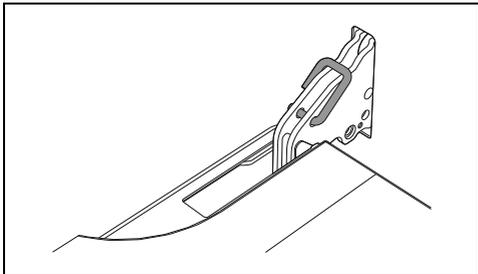
2. Grasp the door on both sides with both hands, lift it so that it forms an angle of around  $30^\circ$  and remove it.
