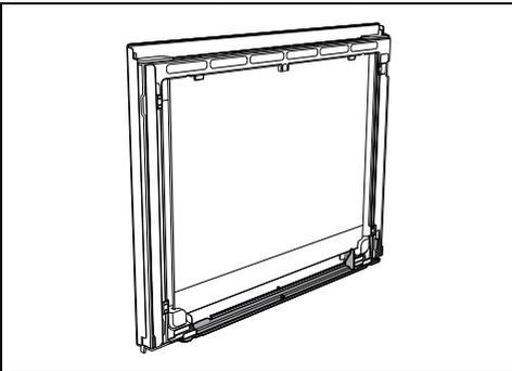
4. Place the internal glass panel back onto the brackets after cleaning. Make sure that you centre and then insert the 4 pins firmly into their housings on the door with the help of
