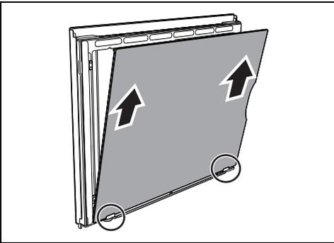
3. After removing the inner glass, it is possible to access the drip catcher strip.
