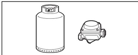
Use a pressure regulator and make the connection on the gas cylinder following the guidelines set out in the standards in force.
