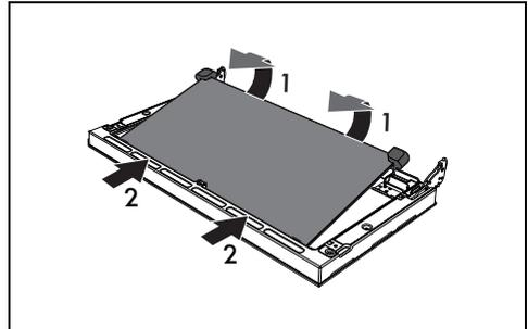
4. Replace the intermediate glass panels after cleaning.
