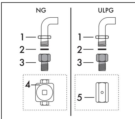
Carefully screw the connector 3 to the appliance's gas connector 1 (1/2" thread
