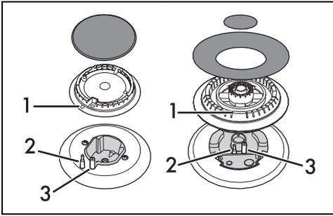
Before lighting the hob burners, make sure that the flame-spreader crowns are correctly positioned in their housings with their respective burner caps. Make sure that the holes 1 in the flame-spreader crowns are aligned with the igniters 3 and thermocouples 2.
