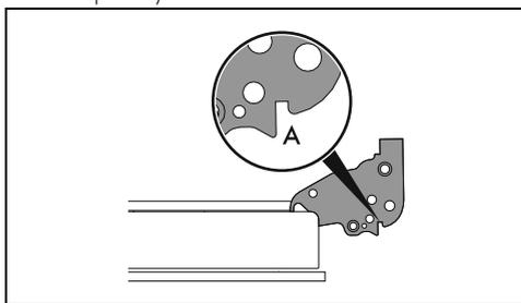
4. Lower the door and once it is in place remove the pins from the holes in the hinges.
