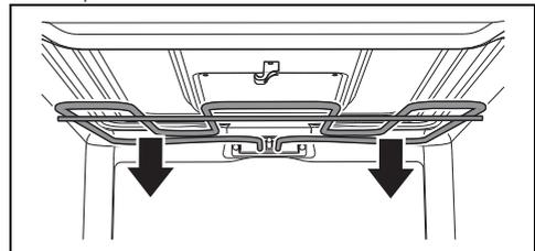
3. When you have finished cleaning, place the heating element back in position and turn the retaining latch to lock it in place.
