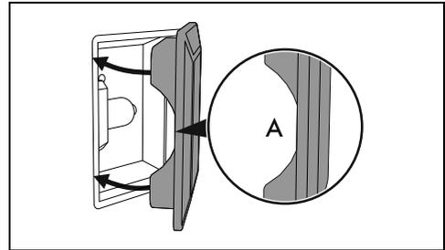
7. Press the cover completely down so that it attaches perfectly to the bulb support.
