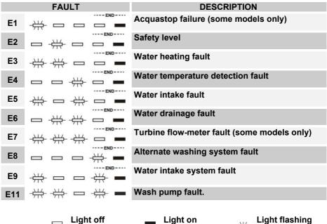
If an alarm occurs, the machine stops the current program and indicates the fault.
