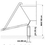
If a horizontal drain extension hose is used (for a maximum 3 m), the drain hose can be placed at a maximum height of.**85 cm** from the ground.
