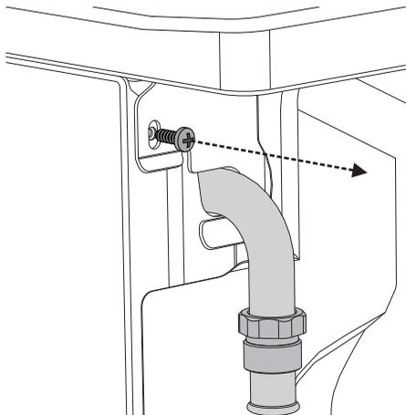
2. Attach the chain to the cooker with the screw just removed.
