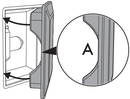
7. Press the cover completely down so that it attaches perfectly to the bulb support.
