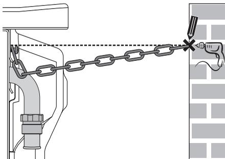
5. Drill the hole and insert a wall plug.
