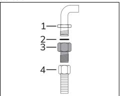
Carefully screw the hose connector 3 to the appliance's gas connector 1 (1/2" thread ISO 228-1), placing the seal 2, provided, between them. Apply insulating material to the thread of connector 3 and then screw the steel hose 4 onto the connector 3.
