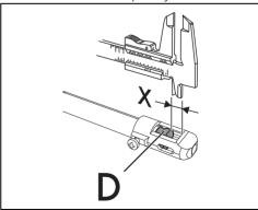
10. Move the Venturi tube "D" to adjust the air flow until distance "X" is reached as indicated in the paragraph (see Table "Burner and nozzle characteristics" -
