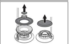
Before lighting the hob burners, make sure that the flame-spreader crowns are correctly positioned in their housings with their respective burner caps. Make sure that the holes in the burners are aligned with the igniters and thermocouples. Also ensure that the flame-spreader crowns are correctly engaged in the burner holes.
