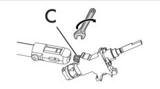
Use a spanner to remove the nozzles "C" and install the new ones for the required gas supply, following the indications given in the relevant table (see "Gas types and countries").
