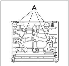
Screw the fixing brackets into the dedicated holes to properly fasten the hob to the built-in structure.
