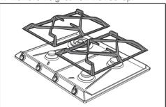
2. Remove the flame-spreader crowns and relative burner caps.
