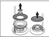
Before lighting the hob burners, make sure that the flame-spreader crowns are correctly positioned in their housings with their respective burner caps. Make sure that the holes in the burners are aligned with the igniters and thermocouples. Also ensure that the flamespreader crowns are correctly engaged in the burner holes.
