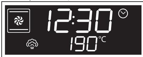
3. While the indicator light
