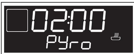
5. Two minutes after the Pyrolytic cycle starts, the
