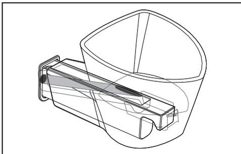
4. Pour the descaling solution into the funnel.
