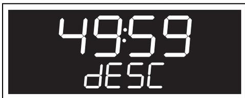
After completion of the descaling process, the appliance sounds an acoustic signal and the display shows the request to drain the descaling solution.
