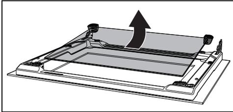
Note: In some models, the intermediate glass unit consists of two panes.
