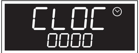
1. Press temperature knob to start adjusting the current time (e.g. "12:30").
