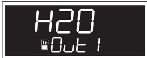
7. Press the temperature knob to drain the water from the reservoir into the deep pan.
