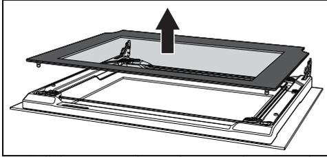
5. Pull the intermediate glass unit downwards from the door and then lift it upwards.
