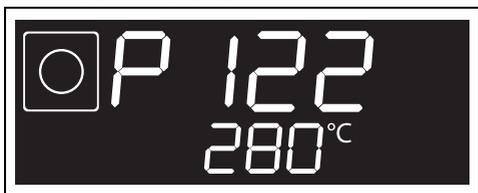
2. Press the temperature knob to confirm the function.
