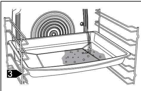
10. Wait for the end of the exhaust flow (check that both level indicator lights
