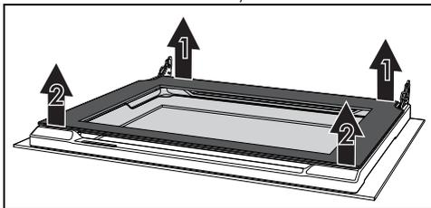
3. Release the front pins following the movement indicated by the arrows 2
