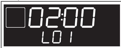
3. Turn the temperature knob to set the duration of the Pyrolytic cycle from a minimum of 2 hours to maximum of 3 hours.
