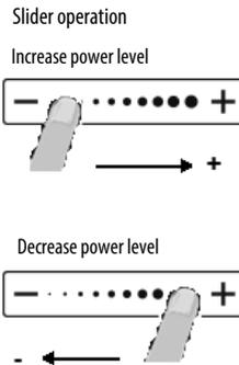
After switching the hob on, activate the required cooking zone by pressing the corresponding circular button and place the pot on the zone. With the Slider control it is possible to select the required power level, from min. 0 to max. 9, or booster “P” if available.
