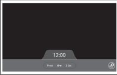
To deactivate the controls lock, press and keep the key icon pressed for 3 seconds; an animation indicates that deactivation is in
