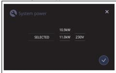
Use your finger to scroll through the available power settings, which can be selected in 0.1 kW steps. (Eco-Logic Advance function).
