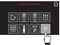
2. Enter the required duration of the cleaning cycle (for example 2 hours and 30 minutes: first touch the minutes box, then the numbers 3 and 0).
