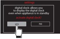
When no appliance function is active, the display will show the current time in digital format.
