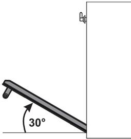
3. To reassemble the door, put the hinges in the relevant slots in the oven, making sure that grooved sections **A** are resting completely in the slots. Lower the door and once it is in place remove the pins from the holes in the hinges.
