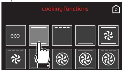
3. The display will show the new function chosen, the preset temperature, the current time and the progress in reaching the new temperature.
