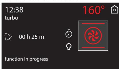
6. Wait for the buzzer to indicate that the time has finished. The symbol
