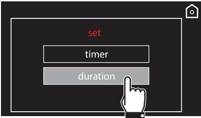
**i** The duration of the timer can be from a minimum of 1 minute to a maximum of 13 hours.
