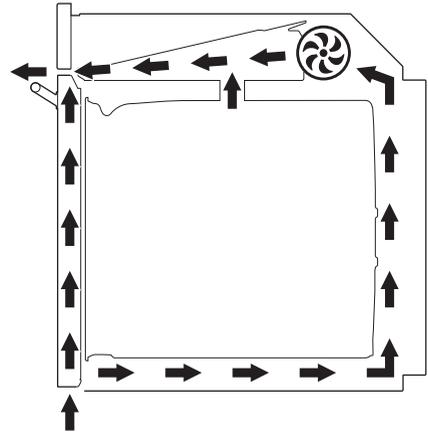
The fan cools the oven and comes into operation during cooking.
