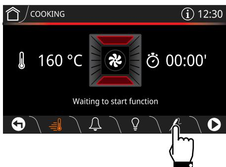
6. Scroll through the **Target temperature** values and select the required temperature (for example "80°C").
