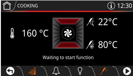
After pre-heating, a buzzer will sound and a message will appear on the display to indicate that the food can be put in the oven.
