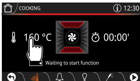
2. Scroll through the values and select the required cooking temperature (for example "180°C").
