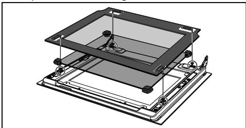
9. Be sure to fit the 4 pins of the inner glass well into their seats on the door.
