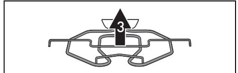
Put the pizza stone base back in place, pushing it in until it hits the back of the oven, and push it down so that the heating element plate is embedded into the base itself.
