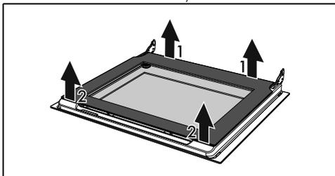
3. Release the front pins following the movement indicated by the arrows 2
