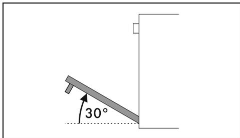
3. To reassemble the door, put the hinges in the relevant slots in the oven, making sure
