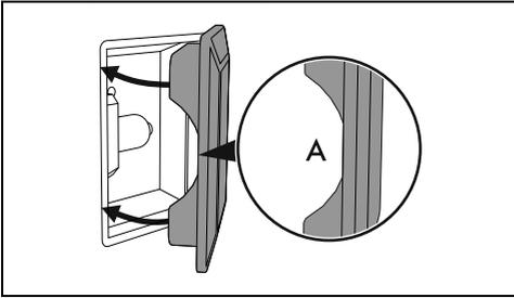
7. Press the cover completely down so that it attaches perfectly to the bulb support.
