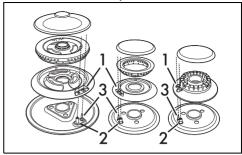
Before lighting the hob burners, make sure that the flame-spreader crowns are correctly positioned in their housings with their respective burner caps. Make sure that the holes 1 in the flame-spreader crowns are aligned with the igniters 3 and thermocouples 2. Also ensure that the flame-spreader crowns are correctly engaged in the burner holes.
