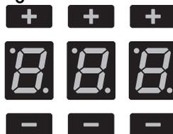
The controls for setting the independent timer and the timer for the cooking zones are located in this area.
