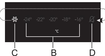
To activate the intensive freezing (freezer boost) function, press the **A** key several times until the symbol **C** lights up.
