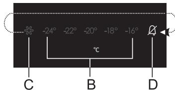
If the temperature inside the appliance is too high, acoustic alarm will be activated (**intermittent tone**) and the **D** symbol will flash.
