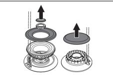
Before lighting the hob burners, make sure that the flame-spreader crowns are correctly positioned in their housings with their respective burner caps. Make sure that the holes in the burners are aligned with the igniters and thermocouples. Also ensure that the flame-spreader crowns are correctly engaged in the burner holes.
