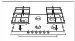
2. Lay the centre grid engaging the notches in the teeth of the lateral grids.
