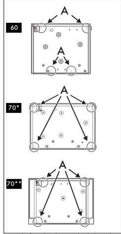
Screw the fixing brackets into the dedicated holes to properly fasten the hob to the built-in structure.
