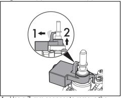
Use a 7-mm spanner to remove the nozzle and replace it with the new one for the required gas supply, following the indications given in the relevant tables (see "Gas types and Countries").
