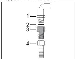
Carefully screw the hose connector 3 to the appliance's gas connector 1 (½" thread ISO 228-1), placing the seal 2, provided, between them. Apply insulating material to the thread of connector 3 and then screw the steel hose 4 onto the connector 3.
