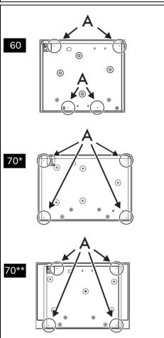
Screw the fixing brackets into the dedicated holes to properly fasten the hob to the built-
