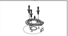
9. Remove the seals from the plugs and thermocouples of each burner.
