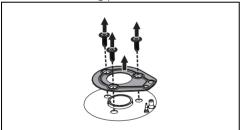
9. Remove the seals from the plugs and thermocouples of each burner.
