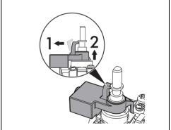
4. Use a 7-mm spanner to remove the nozzle and replace it with the new one for the required gas supply, following the
