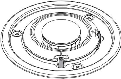
Refit the flame-spreader crowns making sure that they are correctly positioned in their housings with their respective burner caps.
