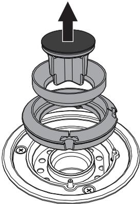
3. Pull the knobs and the knob bezels upwards to remove them.
