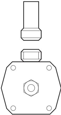
The appliance must be installed with provision to allow the gas to be turned off and disconnected for servicing and removal of the appliance as required from the gas supply. Before the appliance is operated make certain all relevant parts are placed in the correct position.
