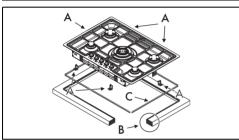
This kind of built-in application needs a milling on the hob top of 3 mm in depth (detail "B" in the picture above). Before positioning the appliance, place the supplied seal (C) on the milling.
