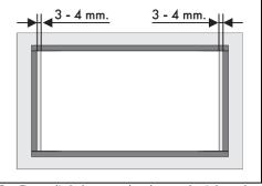
2. Press lightly to make the seal stick to the edge around the hole in the worktop. The front and rear sides of the seal must be flush with the hole.
