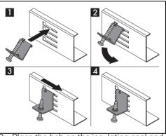
Place the hob on the insulating seal and fix it to the supporting structure using the screws and fastening brackets supplied (A) so that the hob is perfectly level.
