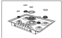
Replace the burner nozzles using a 7mm socket wrench according to the gas to be used (see "Nozzle and burner specification tables").
