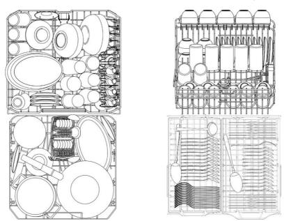
If the bottom basket inserts are of the fold-down type, they should be laid flat for easier loading.
