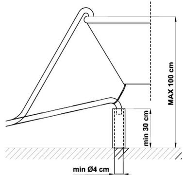
The free end should be positioned at a height of between **30 and 100 cm**, and should never be submerged in water. If a horizontal drain extension hose is used (for a maximum 3 m), the drain hose can be placed at a maximum height of **85 cm** from the ground.
