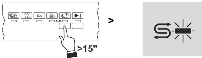
After carrying out the adjustment or displaying the current setting, if you do not touch the button for a few seconds the dishwasher will automatically exit from adjustment mode and return to the standard operating mode.
