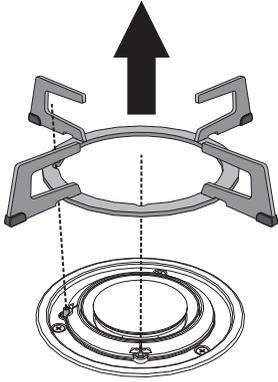
2. Position the new grids on top of the burners.
