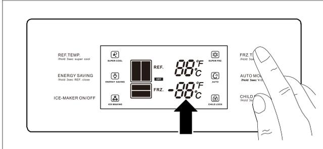
After the temperature adjustment is completed, the new temperature setting will be active for 15 seconds after button was pressed.
