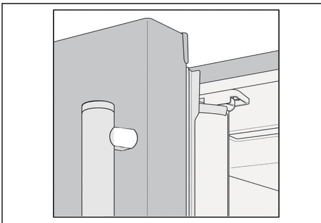
**When closing the left refrigerator compartment door, the door bar folds behind the right refrigerator compartment door, forming a seal between the refrigerator compartment doors.**
