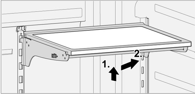
During installation, put the upper end of the fixed leg into the desired slot. Lower the shelf. The lower end of the fixed leg engages into a lower slot.
