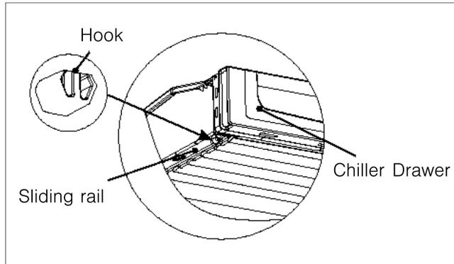
5. Install the drawer by putting the hook into the slots.
