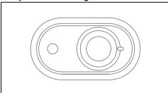
Turn the thermostat knob from position (minimum) to **5** (maximum) depending on the desired temperature.
