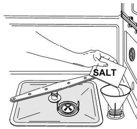
When using water of medium hardness, the regenerating salt container should be refilled after approximately **20 washing cycles**. The salt container can hold approximately **1 Kg** of salt in grains. The container is situated at the bottom of the dishwasher. After removing the lower basket, unscrew the salt container cap by turning it anticlockwise and pour in the salt using the funnel supplied with the dishwasher. Before replacing the cap, remove any salt residues from around the opening.
