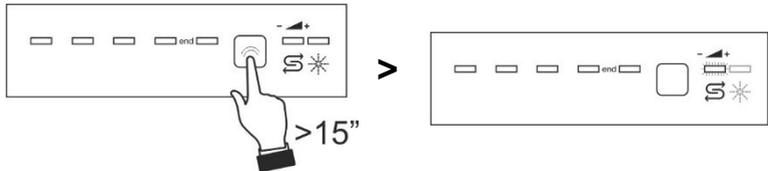
After carrying out the adjustment or displaying the current setting, if you do not touch the button for a few seconds the dishwasher will automatically exit from adjustment mode and return to the standard operating mode.
