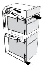
The fan cools the oven and comes into operation during cooking.
