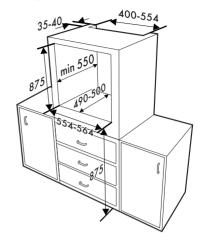
The oven is designed for mounting into any piece of furniture as long as it is heat-resistant. Respect the unit dimensions and the oven overall dimensions for positioning. Depending on the type of installation a slot should be foreseen for ventilating the appliance.
