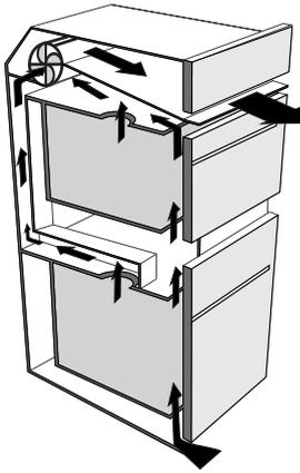
The fan cools the oven and comes into operation during cooking.
