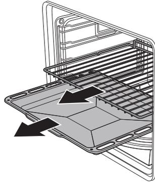
Clean the oven racks with warm water and non-abrasive detergent. Carefully rinse and dry damp parts.
