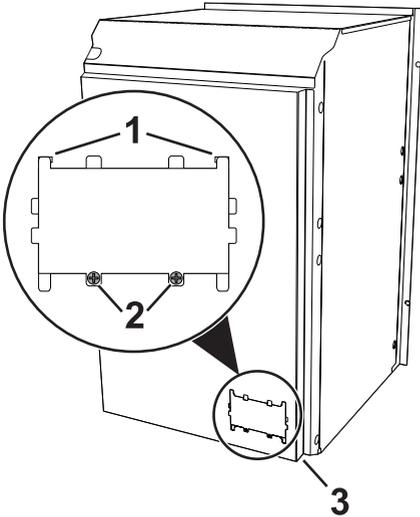
2. Slide the tabs **1** of the terminal board cover out of the grooves;
