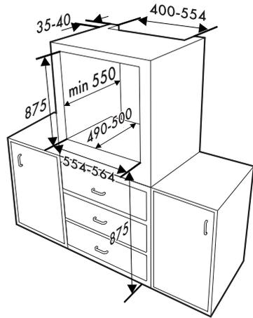
The oven is designed for mounting into any piece of furniture as long as it is heat-resistant. Respect the unit dimensions and the oven overall dimensions for positioning. Depending on the type of installation a slot should be foreseen for ventilating the appliance.
