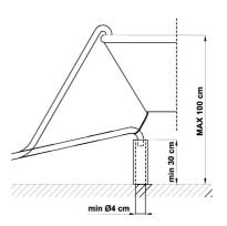
For this purpose, the plastic support is equipped with a hole for tying it to the wall or water tap. The free end should be positioned at a height of between **30 and 100 cm**, and should never be submerged in water. If a horizontal drain extension hose is used (for a maximum 3 m), the drain hose can be placed at a maximum height of **85 cm** from the ground.
