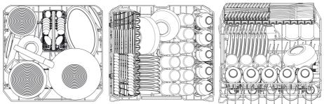
If the bottom basket inserts are of the fold-down type, they should be laid flat for easier loading.
