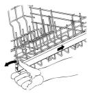
Version B: with adjustment in three positions on both sides. The sides of the basket must always be set at the same height.
