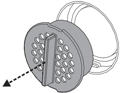
3. Replace the activated charcoal filter with a new one.
