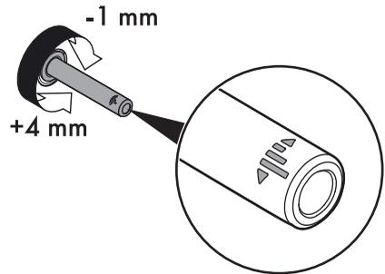
3. Close the door and check that the push-pull mechanism is correctly adjusted.
