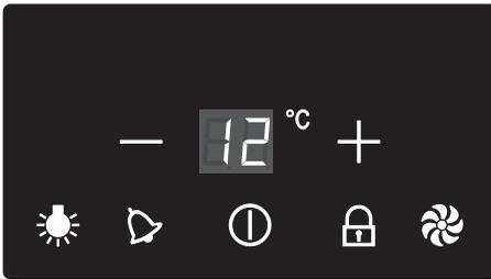
The control panel allows the user to interact with the appliance. Touch the keys with symbols to access the available functions.
