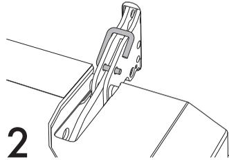
2. Grasp the door on both sides with both hands, lift it forming an angle of around 30° and remove it.
