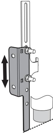
7. Move the bracket onto the wall and mark the position of the holes to be drilled in the wall.
