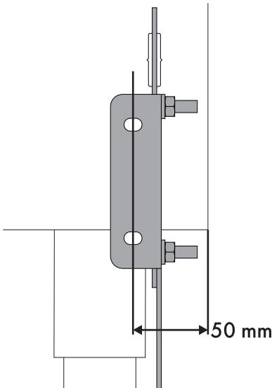
8. After drilling the holes in the wall, use wall plugs and screws to fasten the bracket to the wall.
