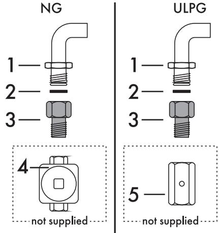
Carefully screw the connector **3** to the appliance's gas connector **1** (1/2" thread BSP), placing the supplied seal **2** between them.
