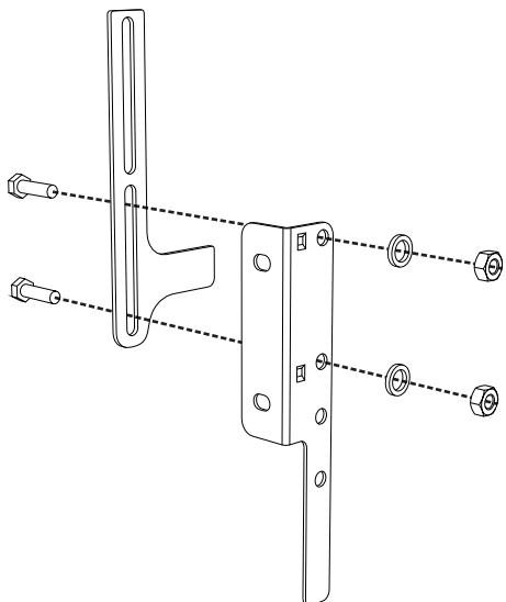
4. Align the base of the hook on the fastening bracket with the base of the slot on the wall fastening plate.
