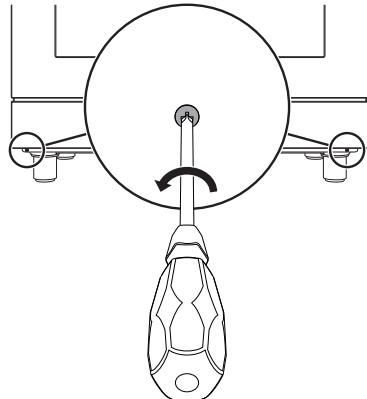
2. Align the front plinth with the corresponding holes on the appliance.
