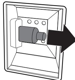
Do not touch the halogen light bulb directly with your fingers, but wrap it in insulating material.
