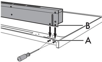
4. Tighten the 4 screws previously loosened.
