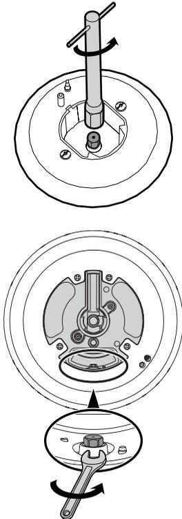
3. Replace the burners in the correct position.
