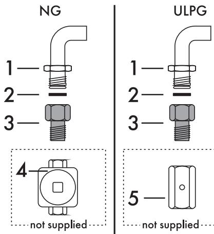
Carefully screw the connector **3** to the appliance's gas connector **1** (1/2" thread BSP), placing the supplied seal **2** between them.
