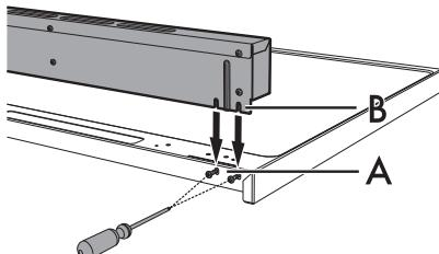
4. Tighten the 4 screws previously loosened.
