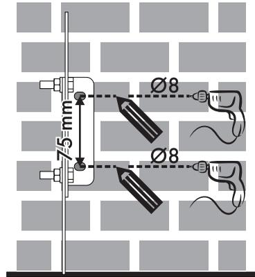
6. Use 50 mm for the distance from the side of the appliance to the bracket holes.
