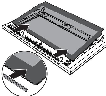
3. Remove the intermediate glass panel by lifting it upwards.
