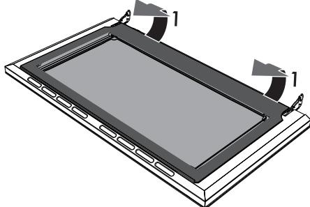
2. Remove the internal glass panel from the front strip (2) to remove it from the door.
