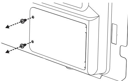
2. Rotate the plate slightly and remove it from its seat.
