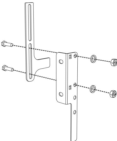
5. Align the base of the fastening bracket so that it reaches the floor and tighten the screws to fix it in position.
