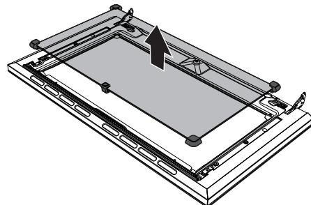
There are 2 intermediate glass panels on the pyrolytic model.
