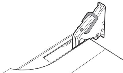
2. Grasp the door on both sides with both hands, lift it forming an angle of around  $30^\circ$  and remove it.
