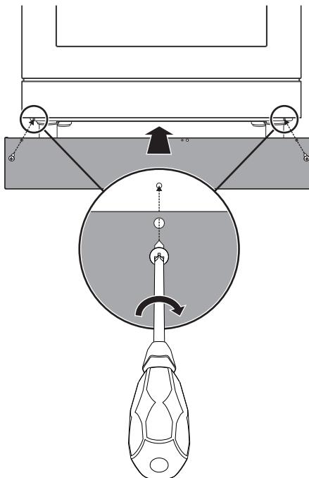
3. Fasten the front plinth to the appliance using the screws that were previously removed.
