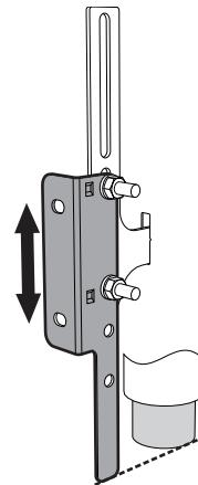
4. Align the base of the hook on the fastening bracket with the base of the slot on the wall fastening plate.
