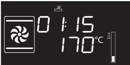
3. A few seconds after having set the required duration, the indicator light stops flashing and timed cooking starts.
