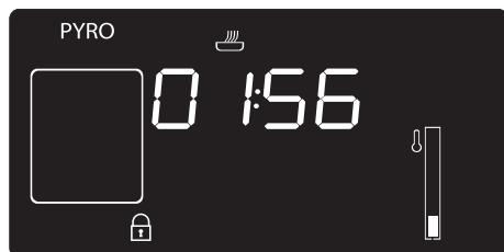
1. The display indicates PYRO or PYRO ECO and the remaining time to indicate that the appliance is carrying out the automatic cleaning cycle.
