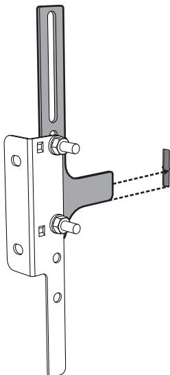
6. The distance from the side of the appliance to the holes in the bracket should be 50 mm.
