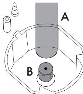
4. If the pressure is 2.75kPa, reassemble the burner and perform the final checks as per this instruction manual.
