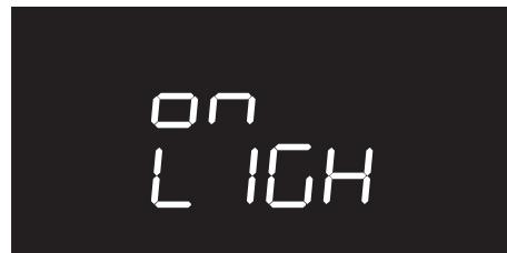
To prevent the appliance from turning off the light automatically after one minute set this mode to OFF.
