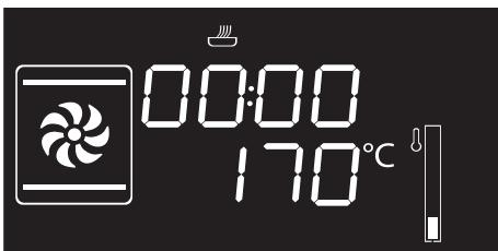
2. Turn the temperature knob to the right or left to set the cooking duration from 00:01 to 12:59. Keep the knob turned to produce a faster increase or decrease.
