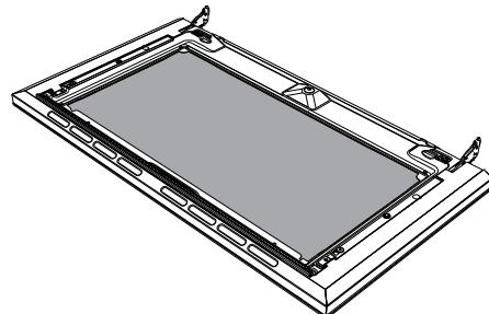
5. When you have finished cleaning, replace the intermediate glass panel into the housing on the door.
