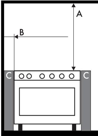
**A** 600 mm (Overhead) measured from the highest part of the highest burner and 750 mm for an exhaust fan.
