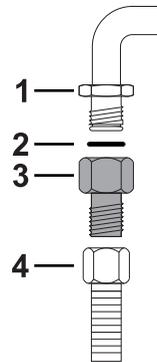
Carefully screw the hose connector **3** to the appliance's gas connector **1** (1/2" thread ISO 228-1), placing the supplied seal **2** between them.
