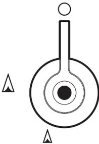
Used for lighting and adjusting the hob burners. Press and turn anti-clockwise to in order to light the relative burners.
