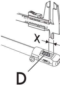
4. Move the Venturi tube "D" to adjust the air flow until distance "X" is reached as indicated in the paragraph (see "Burner and nozzle specifications table" and then secure the tube by means of screw "A").
