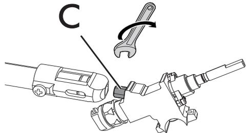
2. Use a spanner to remove the nozzles "C" and install the new ones for the required gas supply, following the indications given in the relevant table (see "Burner and nozzle specifications table").
