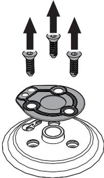
5. Remove the gasket on each burner's thermocouple and igniter.
