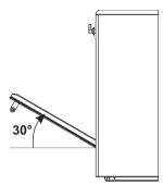
To reassemble the door, put the hinges in the relevant slots in the oven, making sure that grooved sections A are resting completely in the slots. Lower the door and once it is in place remove the pins from the holes in the hinges.
