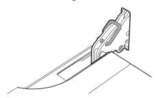
Grasp the door on both sides with both hands, lift it forming an angle of around 30° and remove it.
