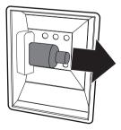
Do not touch the halogen lamp directly with your fingers, but wrap it in insulating material.
