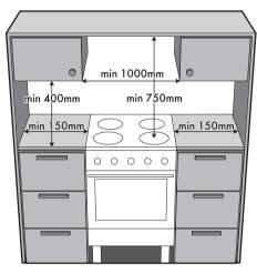
If a hood is installed above the hob, refer to the hood instruction manual to ensure the correct clearance is left.
