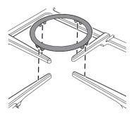
he pan support must be placed on the hob grid as shown in the figure above.
