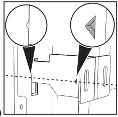
Before tightening the brackets fully to the wall, check that the index on the brackets is at the same height as the index on the back of the appliance. Position the appliance, taking care that the brackets are correctly inserted.
