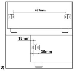
Use the same height on the wall to drill the holes for fastening the brackets. The distance between the centres of the holes is given in the diagram above.
