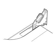
Open the door completely. Insert a pintle into the hole in the hinge. Repeat for both hinges.
