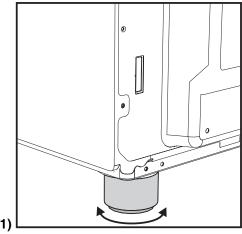
Use the adjustable feet to level the appliance at the required height.
