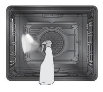
Spray a water and washing up liquid solution inside the oven using a spray nozzle. Aim the spray towards the oven cavity. At the end of this process, close the door and set the cleaning cycle.
