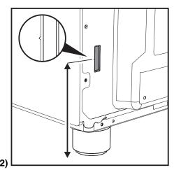
Measure the distance from the index of the opening to the floor.
