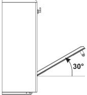
Grasp the door on both sides with both hands, lift it forming an angle of around 30° and remove it.
