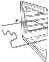
Having prepared the rotisserie rod with the food, position it on the guide frame as shown in the figure.
