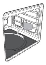
Pour approx. 40 cc of water onto the floor of the oven (as shown in oven. The roof lining can be left the figure). Make sure it does not overflow out of the cavity.
