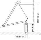
If a horizontal drain extension hose is used (for a maximum 3 m), the drain hose can be placed at a maximum height of.**85 cm** from the ground.
