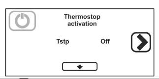
**Set as** "on" = **minimum rinsing temperature as set**, (see boiler temperature above) regardless of intake water temperature; the cycle duration may be a few seconds longer than the nominal length.
