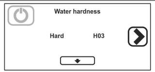
With values over 60°f an external water treatment device must be used and the regeneration frequency must be set on H00.
