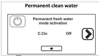
With this option clean water is used for **every** washing. At each cycle, the washing water is completely drained and it is replaced with clean water from rinsing.
