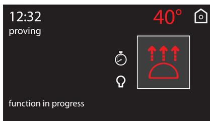
6. While the function is in progress, it is possible to set a timer for a maximum of 4 hours (see “Timer during function”), a proving duration (see “Timed cooking”) or delayed proving (see “Delayed cooking”). Press the symbol to make the required changes.
