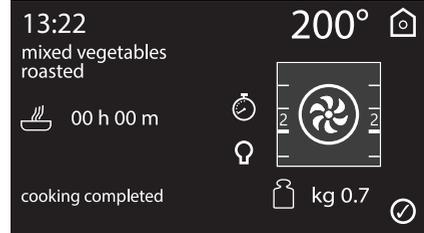
2. To perform a new cooking cycle with the parameters that are already set up, press the
