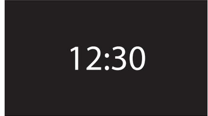
On the first use, or after a power failure, **00:00** will flash on the appliance's display. In order to be able to start any cooking operation, the current time must be set (if the oven is being turned on for the first time, it is also recommended you set the required language).
