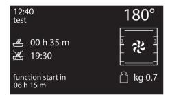
After a few seconds the symbol stops flashing. The appliance waits for the delay start time.
