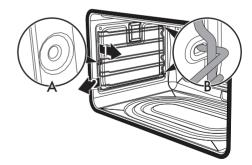
After cleaning, repeat the above procedures to replace the rack/tray support frames.
