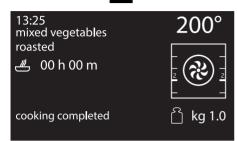
2. Press the control knob to perform cooking with the same parameters currently set (press the knob twice if the buzzer is active). The appliance will restart cooking automatically if it is still at the correct temperature, otherwise it will also restart the preheating stage.
