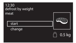
7. Press the control knob again to start defrosting, or select change to further modify the set parameters.
