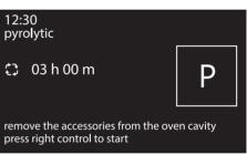
4. Press the control knob to start the pyrolytic cycle.
