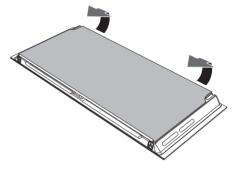
3. Then remove the internal glass panel from the front profile.
