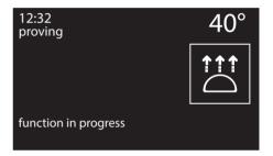
While the function is in progress, it is possible to set a timer for a maximum of 4 hours (see "Timer during function"), a proving duration (see "Timed cooking") or delayed proving (see "Delayed cooking").
