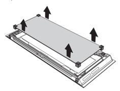
Clean the external glass panel and the panels removed previously. Use absorbent kitchen roll. In case of stubborn dirt, wash with a damp sponge and neutral detergent.
