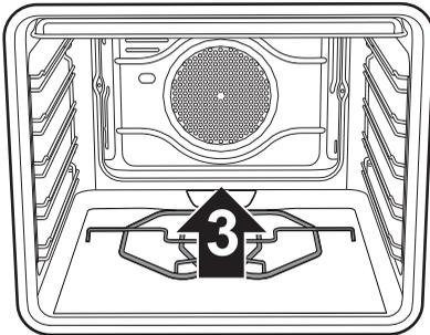
Put the pizza stone base back in place, pushing it in until it hits the back of the oven, and push it down so that the heating element plate is embedded into the base itself.
