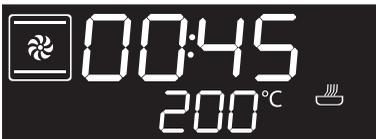
3. A few seconds after the required duration is set, the
