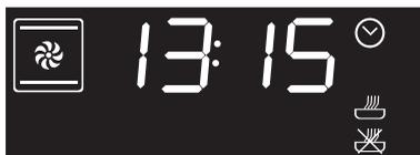
5. At the end of the cooking, STOP flashes on the display and a buzzer will sound that can be deactivated by opening the door or pressing/rotating one of the two knobs.
