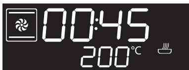
3. Press the programming knob a fourth time. The indicator light
