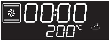
2. Turn the programming knob to set the cooking time (from 00:01 to 13:00). Keep the knob turned to produce a faster increase or decrease.
