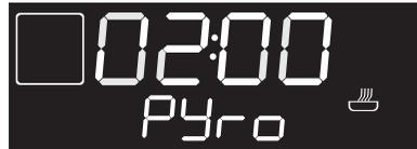
2. The duration of the Pyrolytic cycle will appear on the display.
