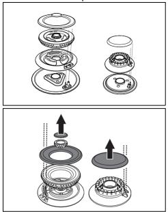
Before lighting the hob burners, make sure that the flame-spreader crowns are correctly positioned in their housings with their respective burner caps. Make sure that the holes in the burners are aligned with the igniters and thermocouples. Also ensure that the flamespreader crowns are correctly engaged in the burner holes.
