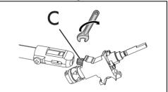
Use a spanner to remove the nozzles "C" and install the new ones for the required gas supply, following the indications given in the
