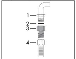
Carefully screw the hose connector 3 to the appliance's gas connector 1 ( $\frac{1}{2}$ " thread ISO 228-1), placing the seal 2, provided, between them. Apply insulating material to the thread of connector 3 and then screw the steel hose 4 onto the connector 3.
