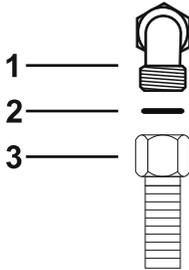
Carefully screw the hose connector **3** to the appliance's gas connector **1** ( $\frac{1}{2}$ " thread ISO 228-1), placing the supplied seal **2** between them. Apply insulating material to the thread of connector **3**, then tighten the steel hose **4** to the connector **3**.
