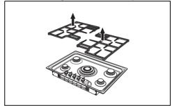
2. Remove the flame-spreader crowns and relative burner caps.
