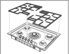
Make sure that the pan supports are simply centred on their respective burners, without forcing them to be raised or tilted. If they are, repeat the positioning procedure.
