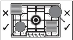
When cooking, to avoid burns, damage to the hob or top, all containers or griddles must be positioned within the perimeter of the hob.
