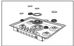
Replace the burner nozzles using a 7-mm socket wrench according to the gas to be used (see "Nozzle and burner specification tables").
