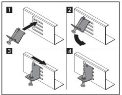
Place the hob on the insulating seal and fix it to the supporting structure using the screws and fastening brackets supplied (A) so that the hob is perfectly level.
