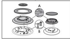
Before lighting the hob burners, make sure that the flame-spreader crowns are correctly positioned in their housings with their respective burner caps. Make sure that the holes 1 in the flame-spreader crowns are aligned with the igniters 3 and thermocouples 2.
