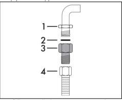
Carefully screw the hose connector 3 to the appliance's gas connector 1 (½" thread ISO 228-1), placing the seal 2, provided, between them. Apply insulating material to the thread of connector 3 and then screw the steel hose 4 onto the connector 3.
