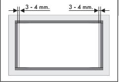
Press lightly to make the seal stick to the edge around the hole in the worktop. The front and rear sides of the seal must be flush with the hole.
