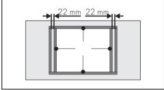
Use light pressure to make the seal stick to the edge around the hole cut in the worktop.
