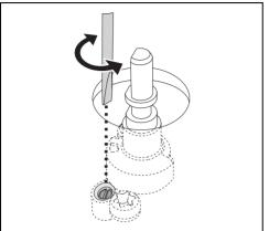
3. Refit the knob and verify that the burner flame is stable.
