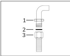
Carefully screw the connector 3 to the gas connector 1 of the appliance, placing the seal 2 between them.
