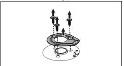
5. Remove the gasket on each burner's thermocouple and igniter.
