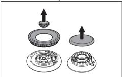
Unscrew the screws under each burner to remove the fixing plate.
