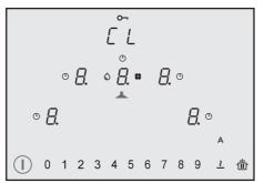
At this point the hob is on but all the cooking areas and the hood are at zero power. The Hob will switch off automatically after 20 seconds if it is not used.
