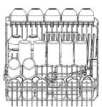
If the bottom basket inserts are of the fold-down type, they should be laid flat for easier loading.
