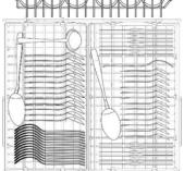
If the bottom basket inserts are of the fold-down type, they should be laid flat for easier loading.
