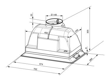
maximum speed (SPEmax): 69 dB(A) Time increase factor (F): 1.5 Measured air flow rate at best efficiency point (Qbep): 300 m<sup>3</sup>/h Measured air pressure at best efficiency point (Pbep): 245 Pa Measured electric power input at best efficiency point (Wbep): 155 W Nominal Power consumption of the light system (WL): 8 W Average illumination of the light on the cooking surface (Emiddle): 100 lux Sound power level at highest setting (Lwa): 69 dB(A)
