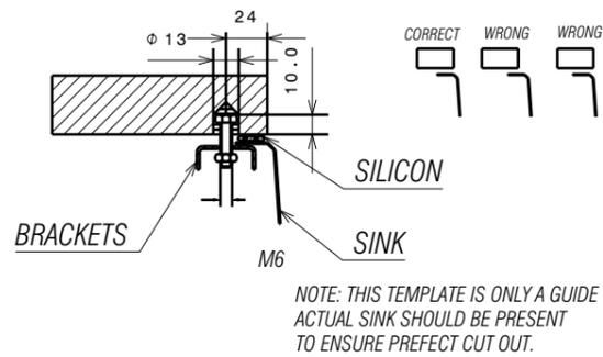
2) Determine placement of clip brackets. Pre-drill holes according to method desired based on countertop material. NOTE: You, the fabricator, may elect to epoxy in the screw or use a brass anchor.
